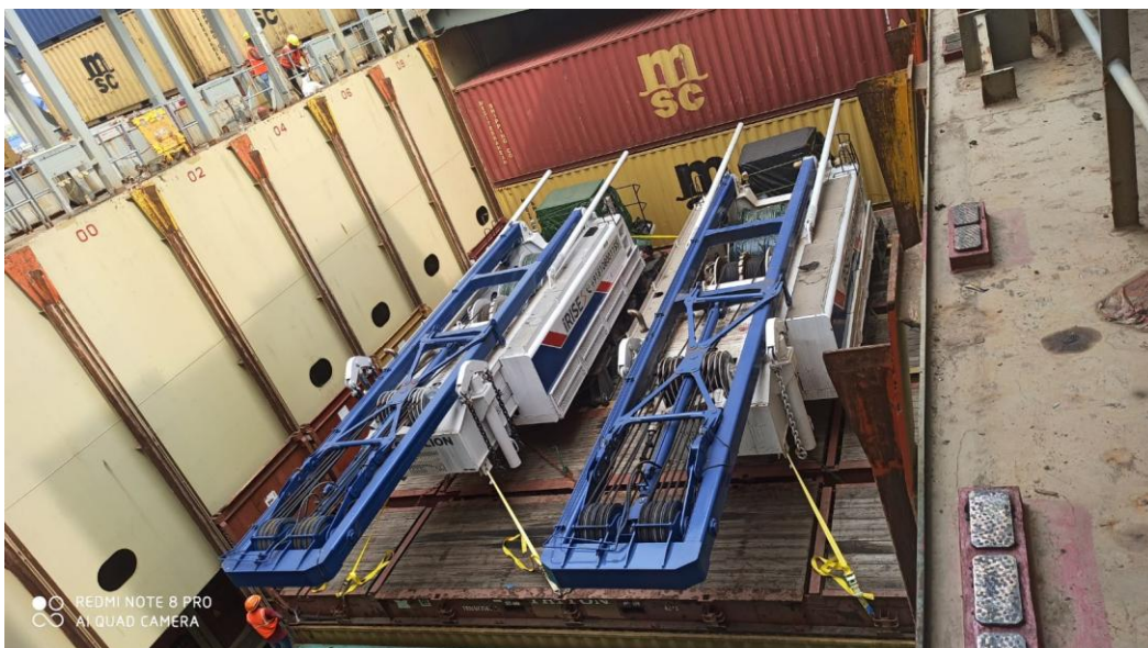
Breakbulk On Container Vessel Weight :- 48 Tons Each, Length :- 14 meter, Width :- 3.30 meter, Height :- 3.10 metere Pkgs :- 2
