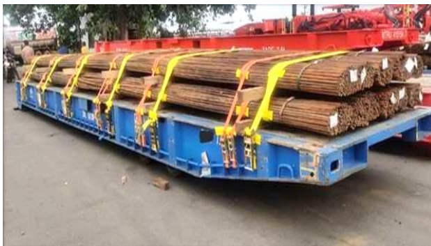
Handling TMT Bars Loaded on 42 Mafi's in Single Shipment, Weight: 2050 Metric Tons, Length: 12.5 meter, POL: India (MBPT) to Ghana (Tema port) West Africa
