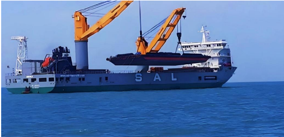
Mid Sea Operation of 750 Metric Ton Single Piece Barge Loading
