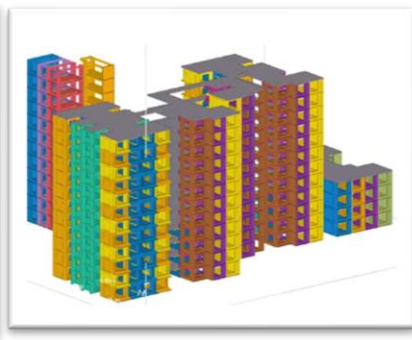
PPVC (Prefabricated Prefinished Volumetric Construction) Modules Construction
