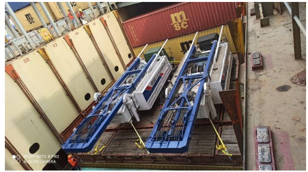
Breakbulk On Container Vessel Weight :- 48 Tons Each, Length :- 14 meter, Width :- 3.30 meter, Height :- 3.10 meters
