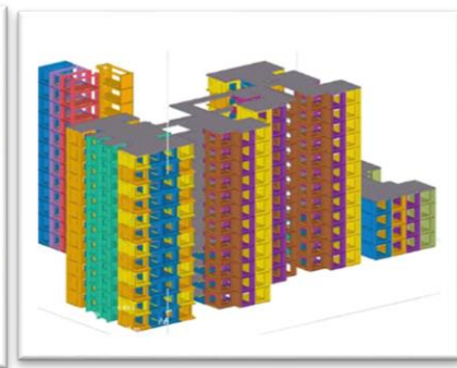
PPVC (Prefabricated Prefinished Volumetric Construction) Modules Construction
