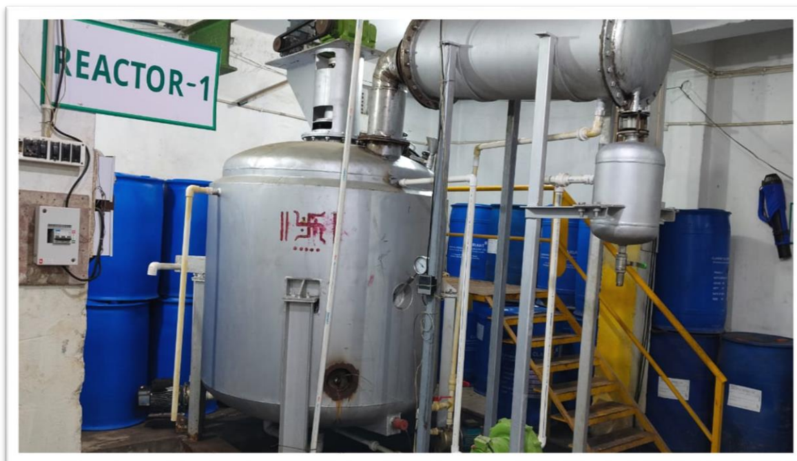
Reactor Vessel with Jacket and Condenser
