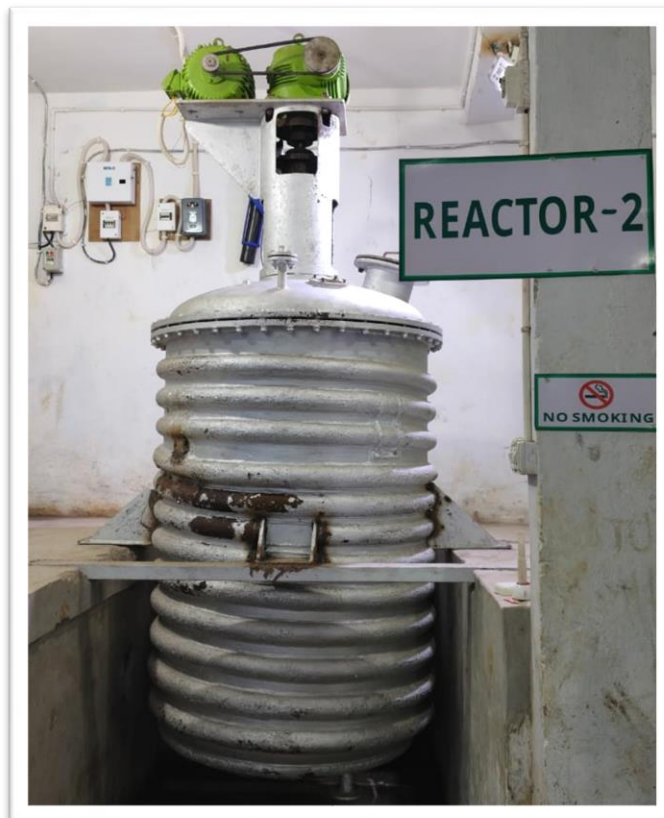
Reactor Vessel – Shell Type
